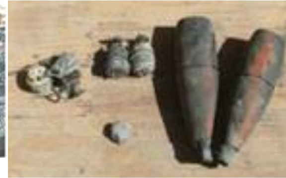
Collected unexploded shell bodies and separated fuzes
