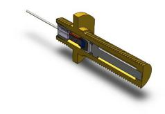
Actuator trials (pressed igniter) ~7 % failure rate
