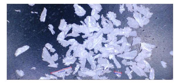
In all cases, CEUK silver azide appears less sensitive than RD1303 and results indicate that coarse silver azide is more sensitive to ESD than fine material; this is despite coarse, non-acicular materials <u>usually</u> being less ESD sensitive than fine explosives and silver azide ESD sensitiveness often being quoted in µJ-levels
