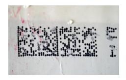
Past: mostly not readable, cells without sharp contours and not aligned columns and rows Today: Printing technologies have developed to such an extent that direct inkjet printing can now be implemented just as well and legibly
