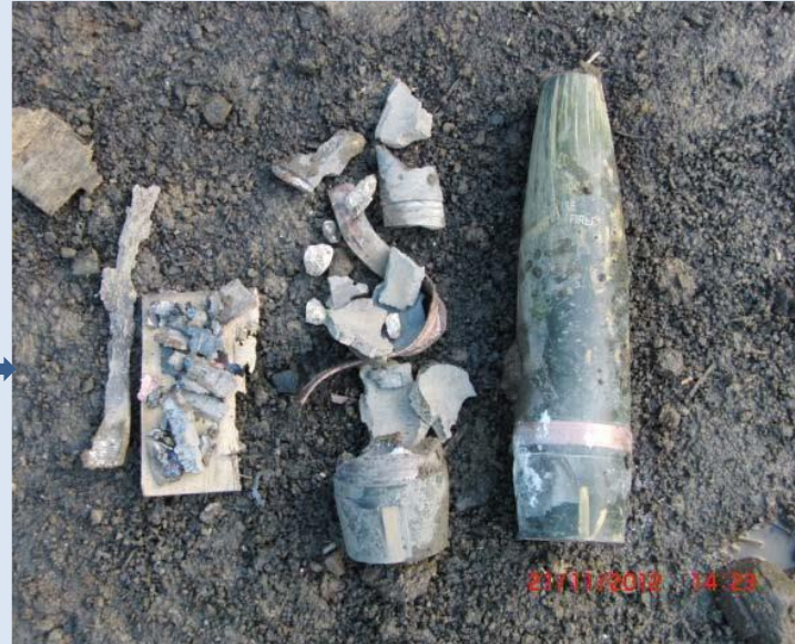
Net Explosive quantity (NEQ) or TNT Eq for each shell is 5kg. The NEQ of three shells detonating sympathetically is 15kg
